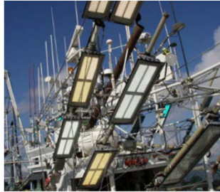
Promoting the introduction of LED fishing lights and energy-saving engines to fishing vessels
