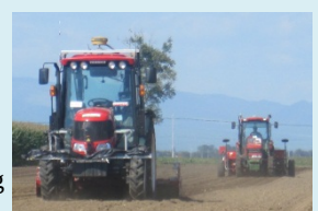
A system for cooperation between unmanned (left) and manned (right) machines
